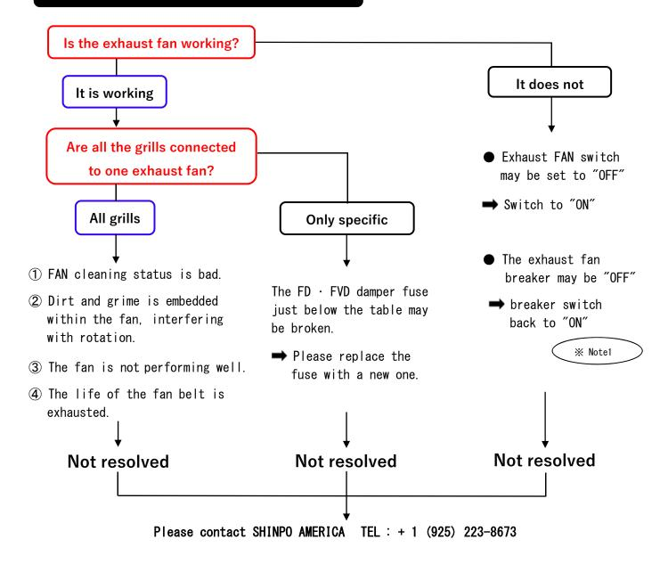
Note 1 - If the circuit breaker is turned "OFF" even if the breaker is turned "ON", there is a possibility of a shock somewhere in the electrical system of the grill. In this case, please contact SHINPO AMERICA. [TEL: +1 (925) 223-8673]
